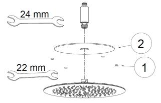
Put the felt covers (1) and the protection gasket (2) supplied on the upper shower head surface. Then, screw the kit to the shower head using a 24 mm wrench and a 22 mm wrench. The gasket (2) does not penetrate dust and/or air inside the cavity between the ceiling and the false ceiling as well as makes soundproof the area. The felt covers (1) protect the false ceiling from any possible scratches during the screwing process.
