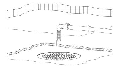
When the installation is completed, make sure that the shower head is perfectly stick to the false ceiling. This installation is the ideal solution for shower heads of huge dimensions and for any shower head with G 1/2 swivel.
