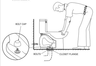
7 INSTALL TOILET SEAT Install toilet seat in accordance with manufacturer's directions.
