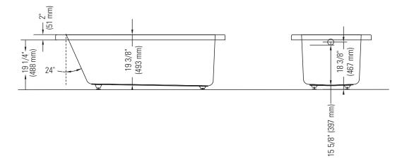
\*A bathtub fitted with back jets can cause the pump to protrude by approximately  $3^{\prime\prime}$  from the overall dimension.
